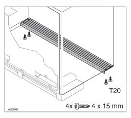
■ Secure the spacer strip to the bottom of the wall unit as well.
